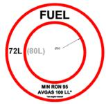
To be stuck around the fuel hole filler. Either with 72 or 80 L depending on the aircraft S/N. Inside diameter: 80 mm
